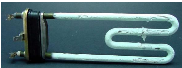
Figure 3b: The effects of limescale: a heating element with limescale deposit
