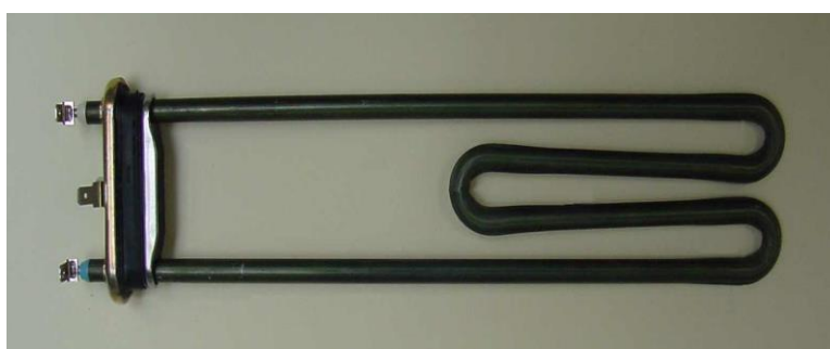
Figure 3a: The effects of limescale: a new heating element
