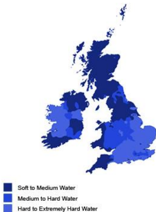
Figure 5: The hardness of water in different areas of the UK (Courtesy of Caterchem UK)
