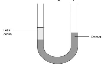
The level of the less dense liquid is above that of the denser liquid.
