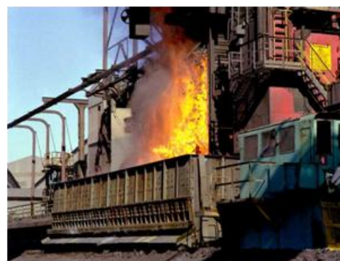
Figure 2 Coal is converted to coke in coke ovens. Thiocyanate ions are a by-product.
