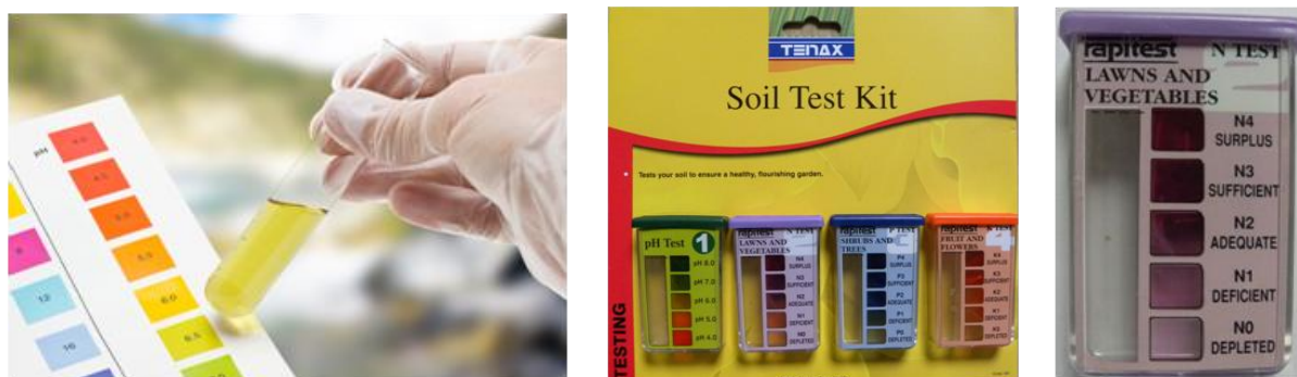
Figure 3 pH test kits can be used to measure soil pH. Other kits are available that also measure the amounts of nutrients available in the soil, for example, nitrogen.
