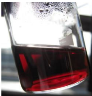
A) Gold nanoparticle colloid B) stabilising effect of citrate ions which prevent agglomeration C) aggregated particles which have fallen out of solution after addition of NaCl
