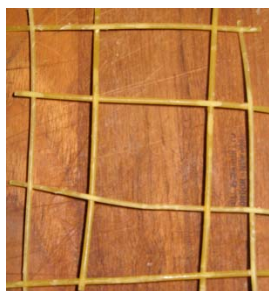
Pasta woven into rigid lattice after softening (not boiling) in hot water
