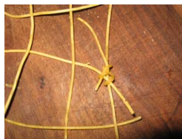
This can be further strengthened by lashing boiled pasta around the joints (like these below!)
