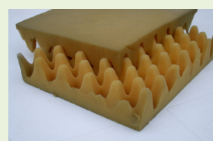
Commensurate surfaces – high friction
