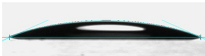
Contact angle 36.5° on an untreated glass slide
