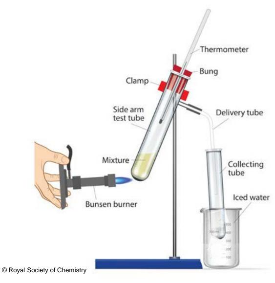
Separating crude oil method 2: side arm boiling tube
