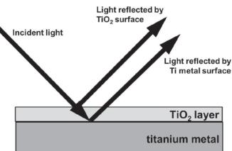
What colour appears is dependent on the thickness of the  $TiO_2$  layer. At a given thickness, certain wavelengths with interfere constructively whilst others will interfere destructively, and so particular voltages (and therefore  $TiO_2$  thicknesses) are associated with particular colours.
