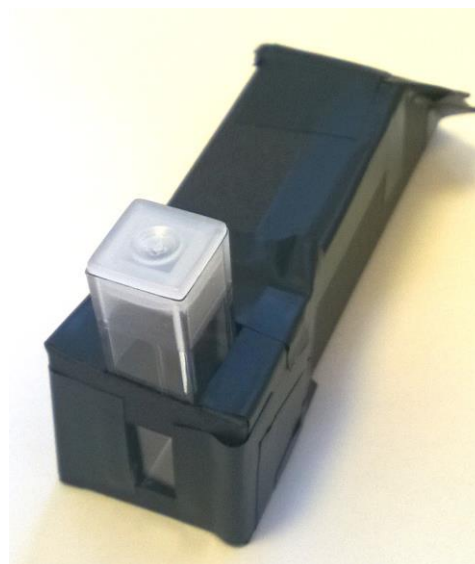
Figure 12: Cuvette adaptor fitted
