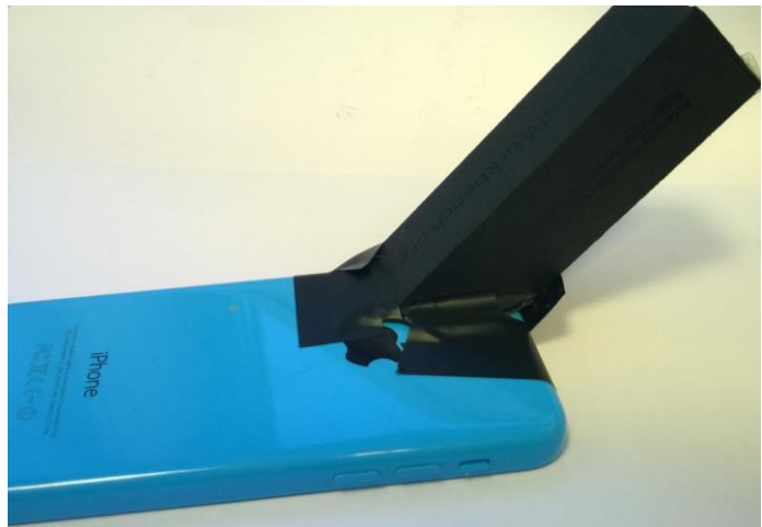
Figure 6: Spectrometer attached to an iPhone
