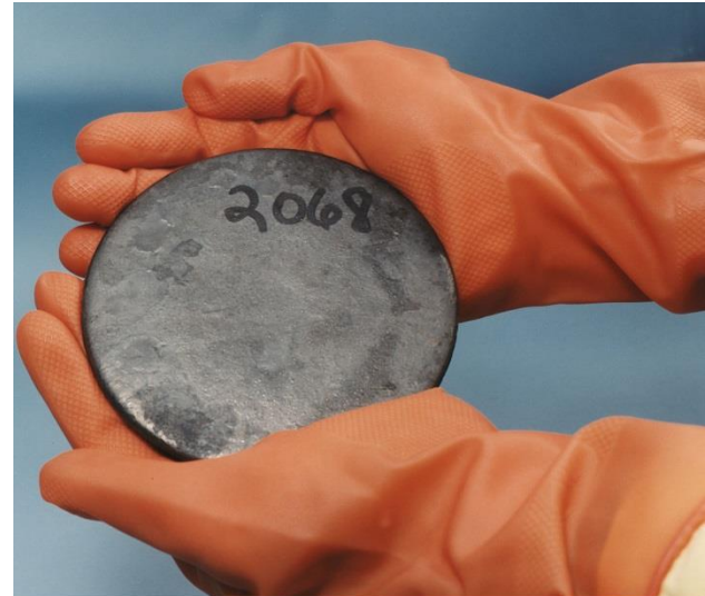
Image credit: A billet of highly enriched uranium (via Wikipedia) or Uranium Enrichment Plant (U.S. Department of Energy via Wiki Commons)
