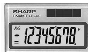
Liquid crystal display in a pocketcalculator
