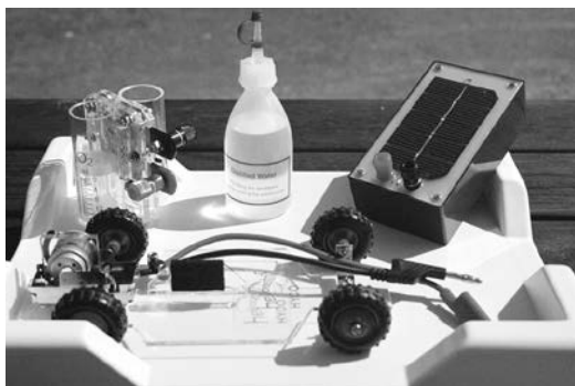
Figure 1: Hydrogen fuel cell used in a model car
