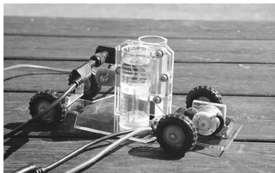
Figure 2: Fuel cell charged up with hydrogen and oxygen
