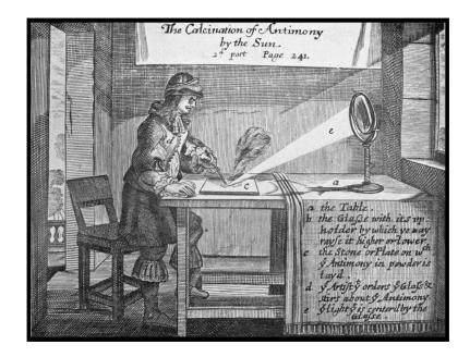
Understanding the proportions in which the elements combine was a crucial step in developing the atomic theory of matter. The picture above shows an experiment performed in the 1660s in which antimony was heated using the sun's rays to form an oxide.
