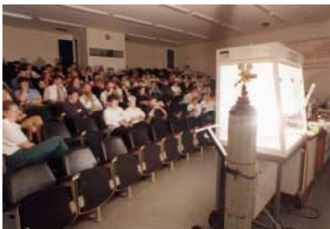
Figure 3. Use of portable fume cupboard to demonstrate ignition of barium perchlorate and magnesium powders.
