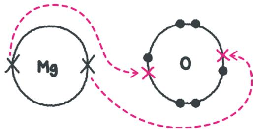
During **ionic bonding** the atoms form ions by **gaining or losing electrons** to obtain a full outer shell. Magnesium loses two electrons and oxygen gains two electrons, leaving  $Mg^{2+}$  and  $O^{2-}$ .
