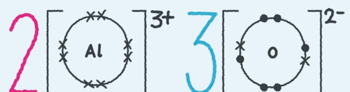
The large numbers in this diagram are multipliers. They mean that there are two aluminium ions for every three oxygen ions.
