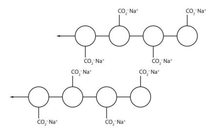
When sodium alginate is put into a solution of calcium ions, the calcium ions replace the sodium ions in the polymer. Each calcium ion can attach to two of the polymer strands. This is called cross-linking and can be represented like this:
