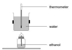
He records the temperature of the water before and after heating it with the ethanol.
