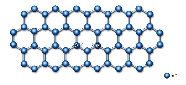
If the C-C bond length in graphene is 0.142 nm, calculate the distance across a single hexagon, labelled distance **AB** on the image. (3 marks)
