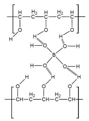
This cross-linking changes the properties of the polymer from a viscous liquid to a far more viscous slime. The slime contains as much as 96% water trapped between the molecules.
