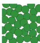
In the liquid state, particles have enough kinetic energy to move freely.
