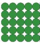
In the solid state, particles only have enough kinetic energy to vibrate around a fixed point.
