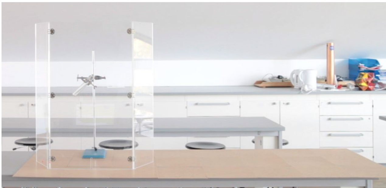
Layout illustrating the protected benchtop with tube pointed along it in the middle of the room © Declan Fleming
