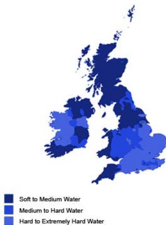
Figure 6: Hardness of water in the UK. The units are mg/l, ie \text{mg dm}^{-3} , of calcium carbonate equivalent (Courtesy of Caterchem UK)
