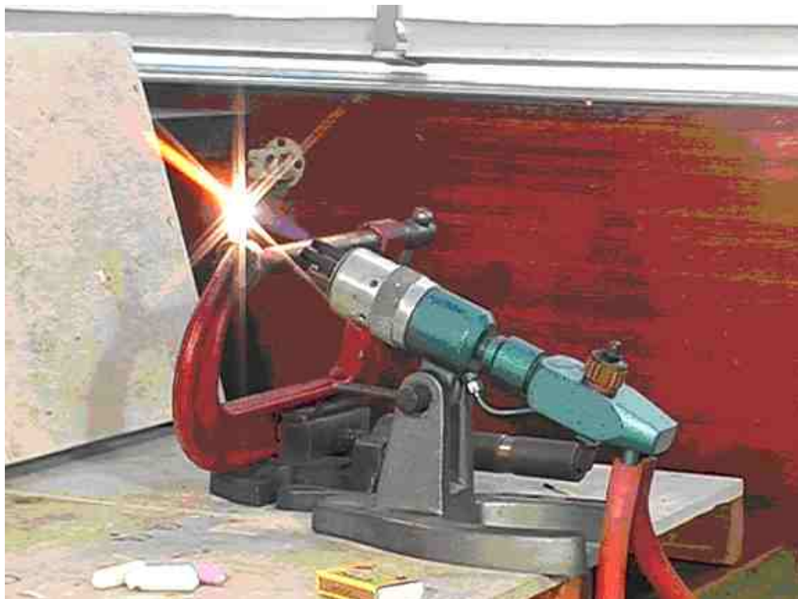
Limelight produced by playing a flame onto a piece of calcium oxide
