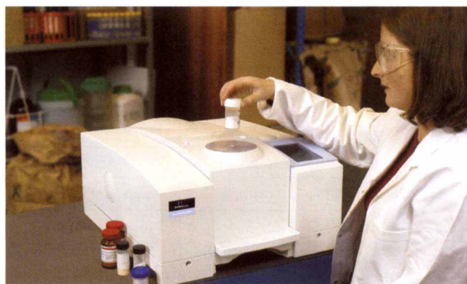
Figure 6 (b) An infrared spectroscopy instrument (Picture reproduced by courtesy of Perkin Elmer.)
