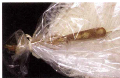
Figure 11 The part of this cellulose nitrate fan that has been kept in a sealed bag has clearly deteriorated more than the exposed part
