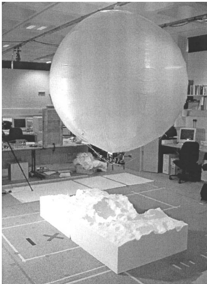
A prototype aerobot helium balloon floats over model Martian terrain. The future of space exploration? Picture used with kind permission of David Barnes, University of Wales, Aberystwyth.
