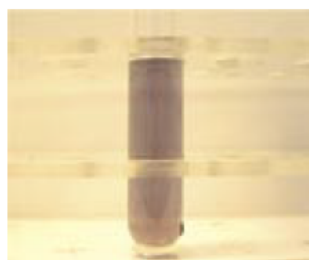
Figure 1 - A is tuned to change colour at slightly below 20°C
