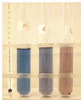
Figure 1 - A is tuned to change colour at slightly below 20°C
