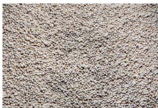
Figure 2 Ammonium nitrate is manufactured on a large scale. Granules are bagged up and distributed to growers. The bag shows the percentage of nitrogen in the fertiliser. Typically it is 34.5%.
