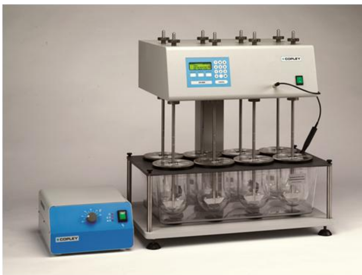
Figure 1 A bank of eight vessels for measuring rate of dissolution using the paddle method. The paddles can be replaced by mesh baskets, allowing the apparatus to be used for the rotating basket method.
