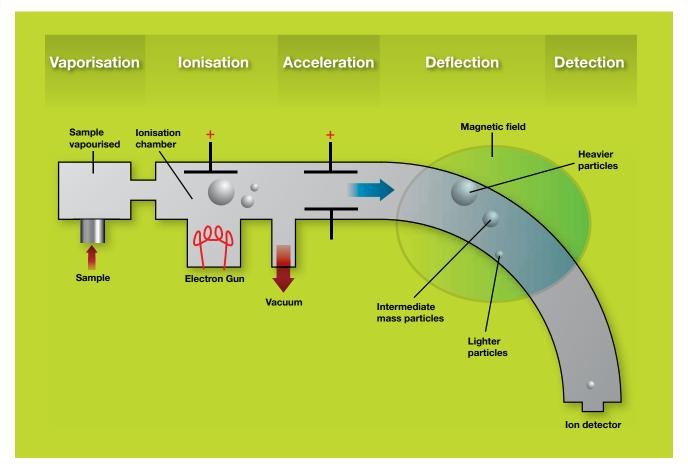
Next, the sample must be **IONISED**. This is achieved by bombarding the sample with **high energy electrons** from an electron gun. These knock off an electron to produce a **positive** ion.
