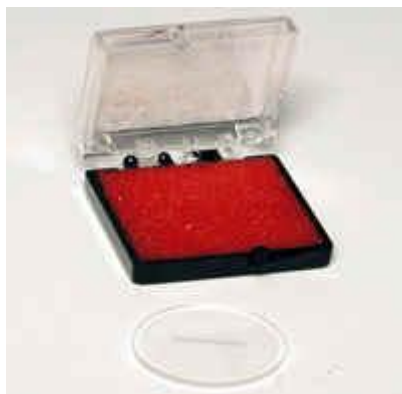
Eyepiece graticule with evenly spaced markings
