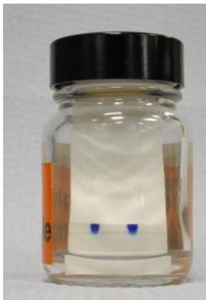
Figure 4. Development tank with plate
