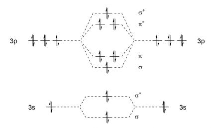
If we complete the diagram with the 8 electrons from each argon atom (a total of 16) we can see that all orbitals (including the anti - bonding orbitals) are occupied, leading to a net bond of 0; i.e. no bond - explaining why we see the noble gases as individual atoms.
