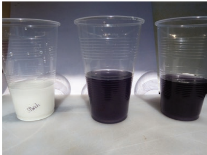
Figure 4 Left = starch solution. Right = iodine solution. Middle = solution for testing when the end point has been reached.
