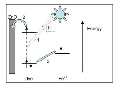
The process starts at the working electrode when the sensitising dye (i.e. the raspberry juice bound to the ZnO layer on the solder wire working electrode) absorbs sunlight (Arrow 1). The energy from the light allows the raspberry dye to excite an electron to a higher energy level and from there the electron is injected into the ZnO semiconductor (Arrow 2) and travels around the circuit to the copper wire where it combines with Cu<sup>2+</sup> ions to make Cu metal.
