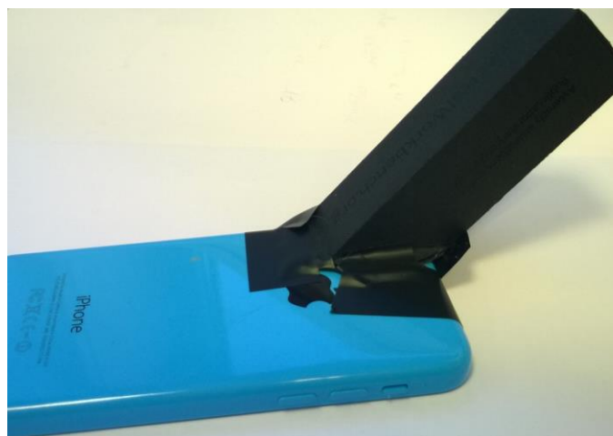
Figure 6: Spectrometer attached to an iPhone
