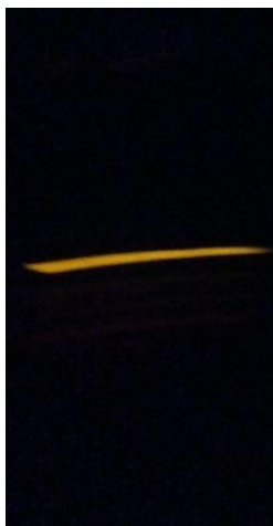
Figure8: spectrum from a sodium flame test
