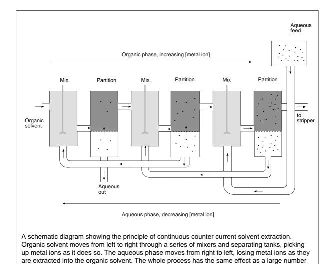
of successive batch solvent extractions. The metal ions are then stripped from the organic solvent
