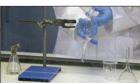
Separation: removing the aqueous layer using a separating funnel, see 02:07.
