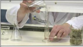
Preparation: combining concentrated hydrochloric acid with 2-methylpropan-2-ol, see 01:08.
