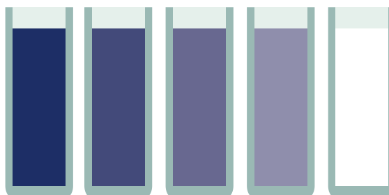
Starch and iodine solutions of increasing dilution used to make the calibration curve
