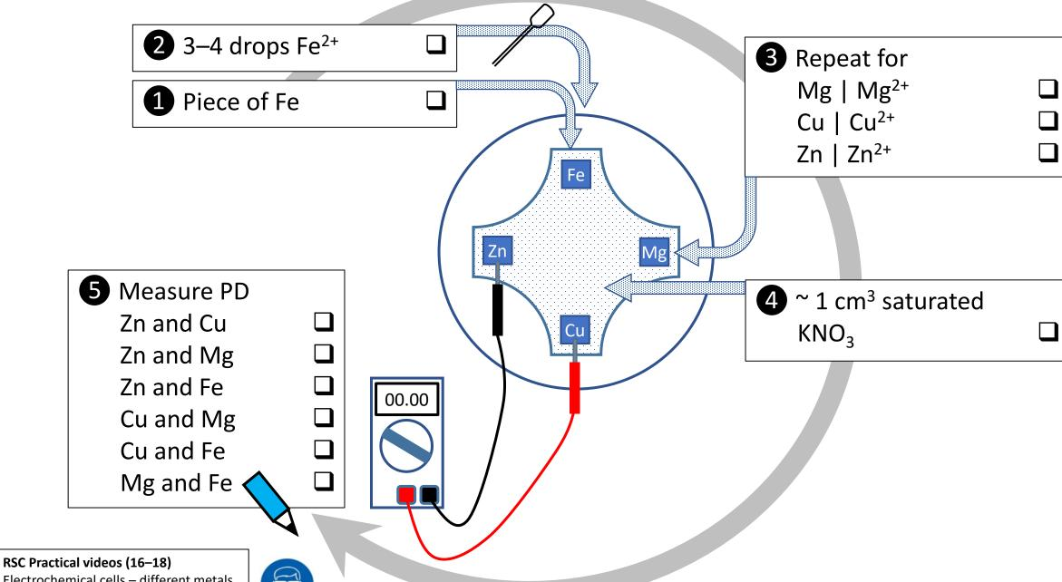
Electrochemical cells – different metals rsc.li/3l0g6sR
